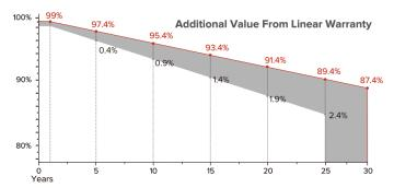
For TOPCON Monocrystalline Modules, the maximum loss of power output from the Peak Power at STC at the end of each year of the Power Warranty Period shall not be greater than (i) 1.0% plus (ii) 0.4% multiplied by the number of years after the end of the first year of the Power Warranty Period (ending with no less than 87.4% at the end of the Power Warranty Period).
