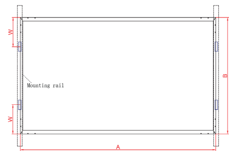
Drawing 4: Mounting rail parallel the short side
